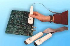
The Advanced Test Module is equally at ease with testing large quantities of boards (production testing) and testing in-circuit single components (repair and diagnostics).
